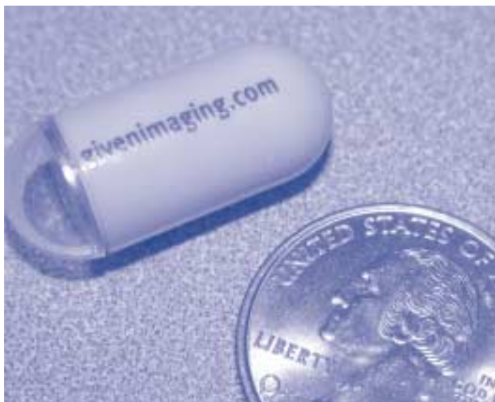
The capsule endoscope (11 x 13 mm) contains a camera, light source, radio transmitter and battery.
