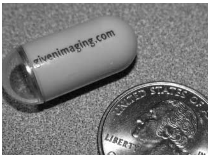
The Capsule Endoscopy Given® Diagnostic Imaging System is a swallowable video capsule which allows physicians to capture images of the small intestine. The capsule—about the length of a quarter—packs a camera, light source, radio transmitter and batteries.
